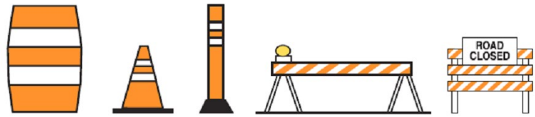
Barrel Cone Tube Barrier Road Closed
