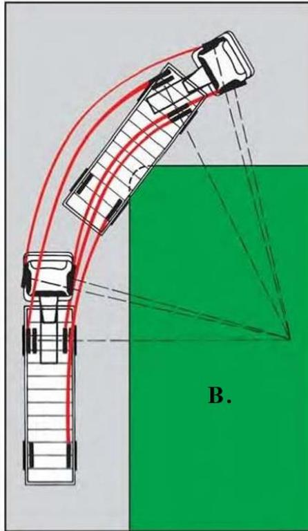
In illustration B, notice the rear wheels of the trailer follow shorter paths than the front wheels of the RV or large non-commercial vehicle.
